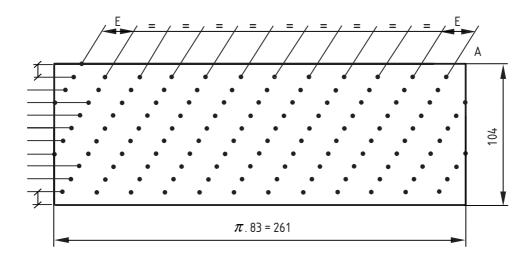
B/B =  $\pi$  83 = 261 mm I = 7 mm The horizontal distance E between tufts is 261/11 = 23,7 mm L = 10 mm
