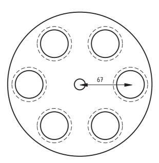
Figure 35 — Holder for jars used in WVP test
