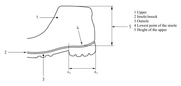
Figure 33 — Measurement of the height of the upper
