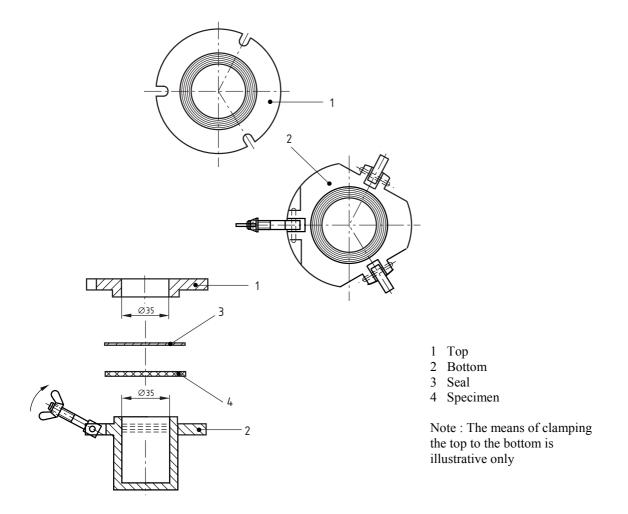
Figure 39 — Apparatus for determination of W.V.A.
