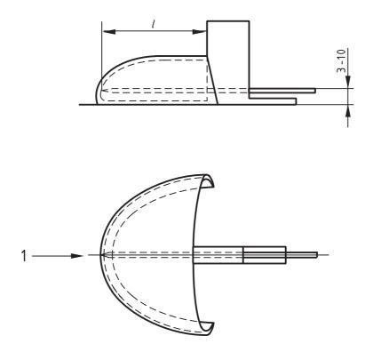
1 Test axis *l* = internal length
