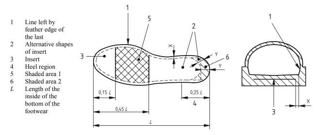
Figure 14 — Determination of dimensions for the insert
