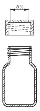
Figure 34 — Jar to be used in WVP test
