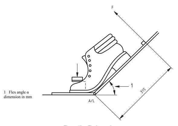
Figure 47 — Flexing angle
