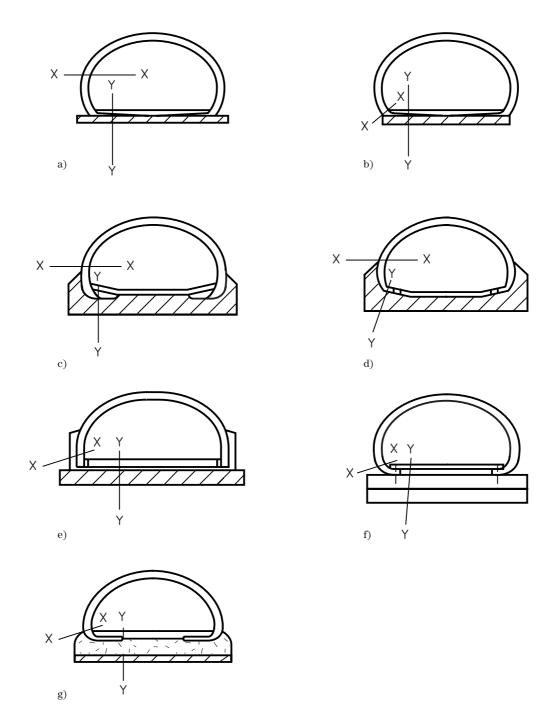
Type a: Conventional lasting, Cemented or moulded outsole having an extended range
