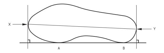
Figure 11 — Test axis for footwear
