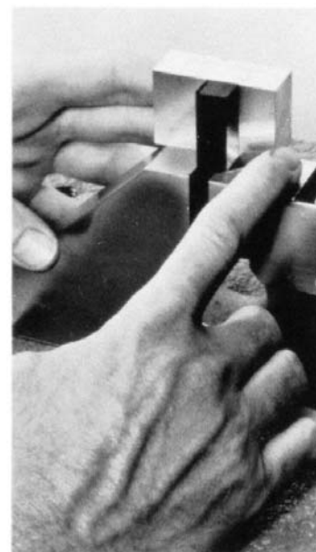
FIG. 4 Jig for Positioning Specimen for Clamping
